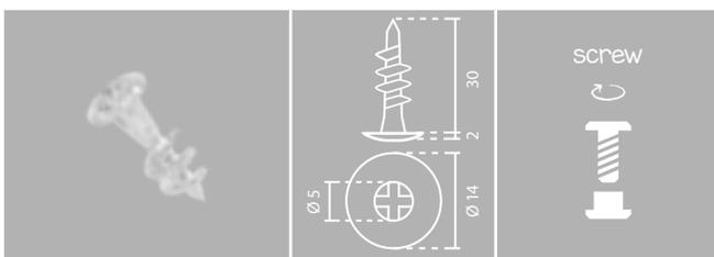
Technical drawing of screw 12.536 showing dimensions: length 30mm, top flange 2mm, hole diameter  $\varnothing 5$ , and base diameter  $\varnothing 14$ . Includes a 'screw' icon with a rotation arrow.
