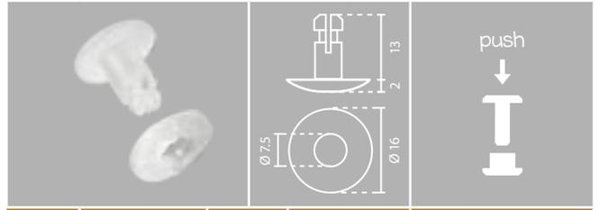
Technical drawing of rivet 12.534 showing dimensions: height 13mm, top flange 2mm, hole diameter  $\varnothing 7.5$ , and base diameter  $\varnothing 16$ . Includes a 'push' icon with a downward arrow.
