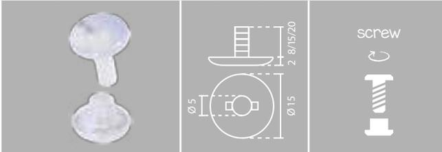
Technical drawing shows a screw with a diameter of  $\varnothing 15$  mm and a hole diameter of  $\varnothing 5$  mm. The length is 8 mm. The drawing also shows a side view with a diameter of  $\varnothing 15$  mm and a height of 2.8/15/20 mm.
