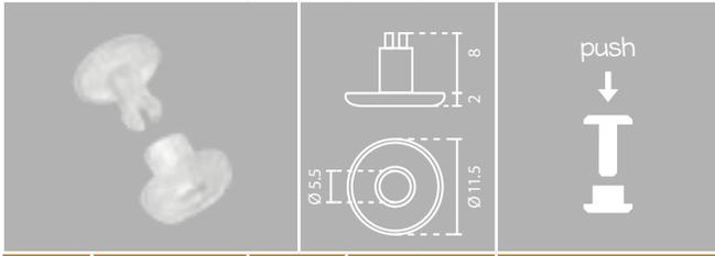
Technical drawing of rivet 12.533 showing dimensions: height 8mm, top flange 2mm, hole diameter  $\varnothing 5.5$ , and base diameter  $\varnothing 11.5$ . Includes a 'push' icon with a downward arrow.
