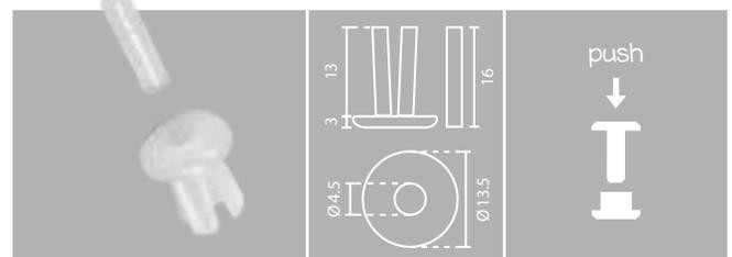
Technical drawing of rivet 12.537 showing dimensions: height 16mm, top flange 3mm, hole diameter  $\varnothing 4.5$ , and base diameter  $\varnothing 13.5$ . Includes a 'push' icon with a downward arrow.
