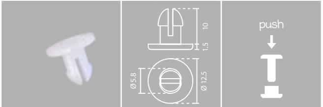
Technical drawing shows a push-in rivet with a diameter of  $\varnothing 12.5$  mm and a hole diameter of  $\varnothing 5.8$  mm. The length is 10 mm. The drawing also shows a side view with a diameter of  $\varnothing 12.5$  mm and a height of 1.5 10 mm.
