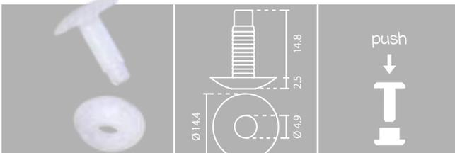
Technical drawing shows a push-in rivet with a diameter of  $\varnothing 14.4$  mm and a hole diameter of  $\varnothing 4.9$  mm. The length is 14.8 mm. The drawing also shows a side view with a diameter of  $\varnothing 14.4$  mm and a height of 2.5 14.8 mm.
