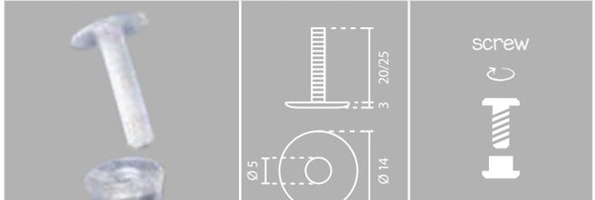
Technical drawing shows a screw with a diameter of  $\varnothing 14$  mm and a hole diameter of  $\varnothing 5$  mm. The length is 20 mm. The drawing also shows a side view with a diameter of  $\varnothing 14$  mm and a height of 3 20/25 mm.
