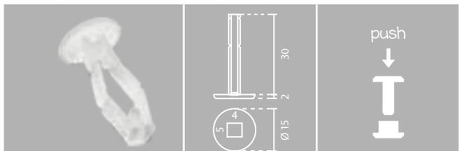
Technical drawing shows a push-in rivet with a diameter of  $\varnothing 15$  mm and a hole diameter of  $\varnothing 5$  mm. The length is 30 mm. The drawing also shows a side view with a diameter of  $\varnothing 15$  mm and a height of 2 30 mm.
